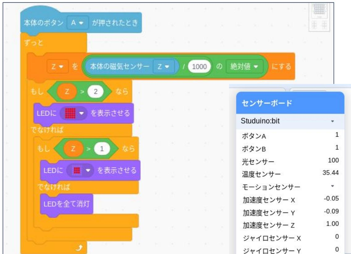
The image shows a Scratch script and a sensor board. The script starts with a 'when button A is pressed' event, followed by a 'loop forever' block. Inside the loop, the Z-axis value of the magnetic sensor is divided by 1000 and its absolute value is taken. Two conditional checks follow: if Z > 2, the red LED is lit; if Z > 1, the red LED is lit and all other LEDs are turned off. The sensor board data on the right shows the Z-axis magnetic sensor value as 2891, which is circled in red.
